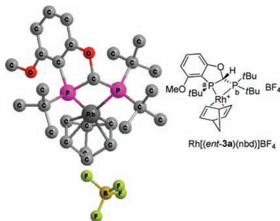
Figure 2. X-ray structure of Rh[( ent - 3a )(nbd)]BF 4 [the H atoms are omitted for clarity, selected bond lengths (Å) 2.281 (Rh–P(a)), 2.337 (Rh–P(b)); selected bond angle (deg) 73.7 (P(a)–Rh–P(b))]
